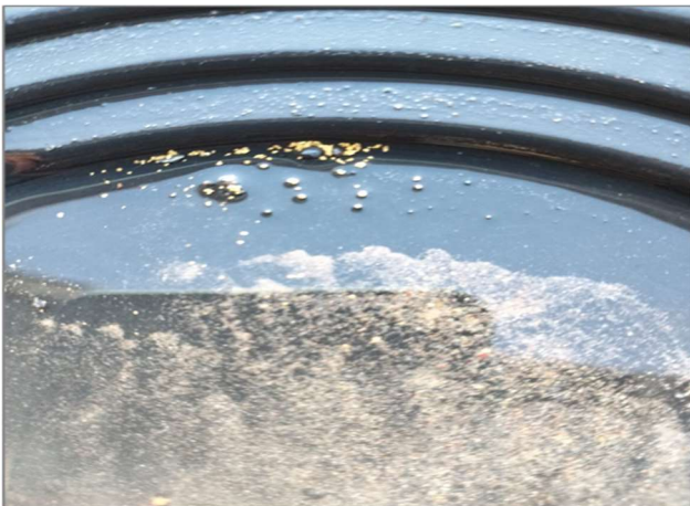
Figure 1. Single pan-concentrate containing 40+ visible gold grains, panned at Camp Oven Creek.
