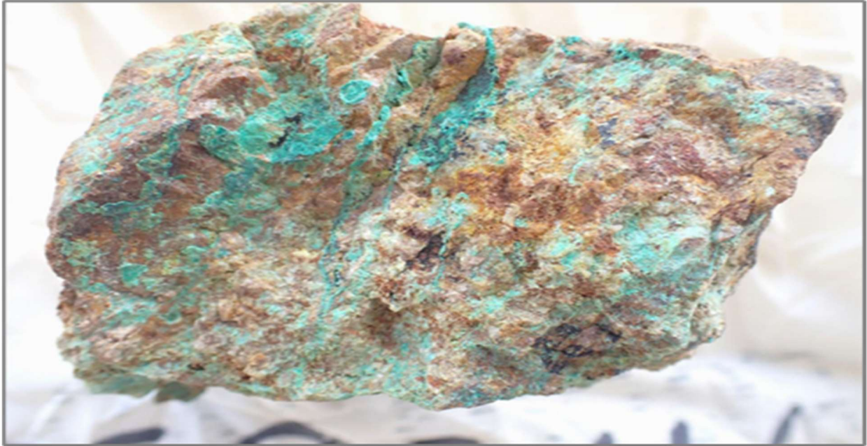
Figure 5. Sample ESS02116 – 774610E 8007802N (63 ppm Ag, 815 ppm Bi, 6.26% Cu, 2090 ppm Pb). Disseminated and stockwork veinlet oxide copper mineralization postdating host cataclastically brecciated granodiorite.
