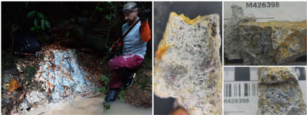
Figure 4 – Mineralization at Cobrasco Central – disseminated bornite-chalcopyrite-chalcocite in rhyolite porphyry (Sample No M426398: 4.77% Cu, 73.7ppm Mo, 11.4ppm Ag).
