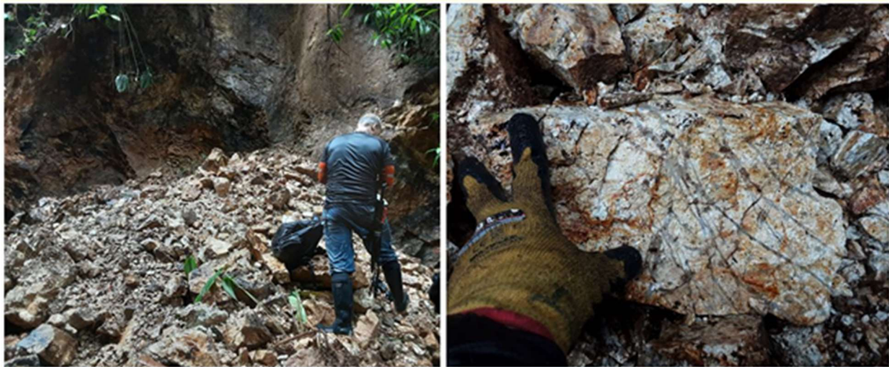
Figure 2: New discovery outcrop in Cobrasco NE, over an area of recent landslide with stockworked quartz-pyrite veining in tonalite porphyry with dominant phyllic alteration (Sample No. L874550: 238ppm Cu, 3.21ppm Mo, 9.7ppm Ag).
