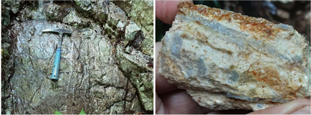
Figure 3: Mo-Cu mineralization at Cobrasco NE- sheeted quartz veins in tonalite porphyry (Sample No. G518018: 927ppm Mo, 3800ppm Cu, 9.7ppm Ag).
