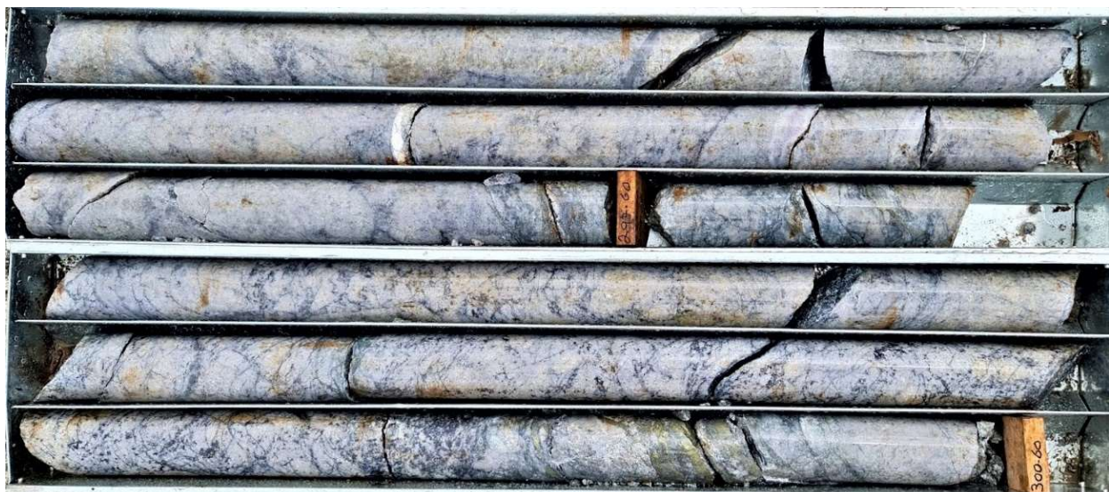
Figure 1. Mineralised quartz diorite porphyry with dominant bornite (dark colour) and lesser chalcopyrite (CDH003 to the current depth of 300.6m, HQ core).
